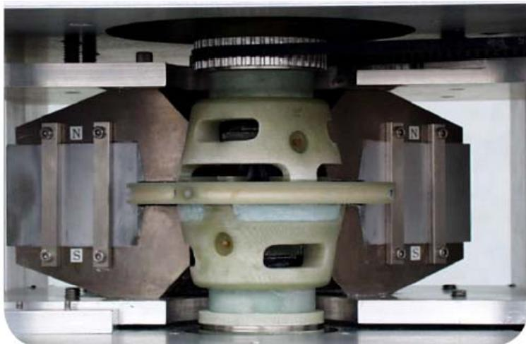
*A rotating magnetic refrigerator developed by Astronautics Corporation of America Ltd. in collaboration with the Ames Laboratory.*
